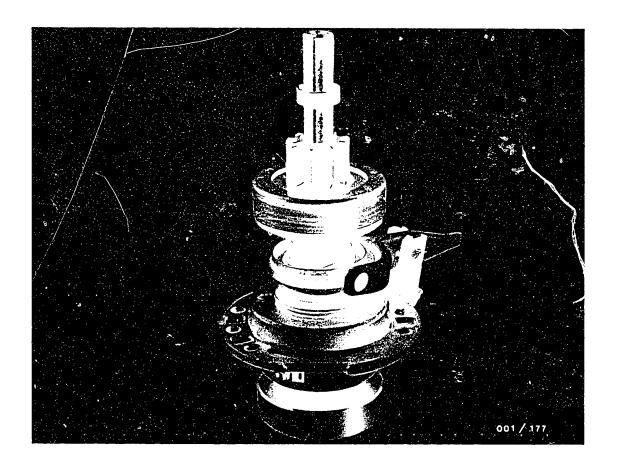
In order to avoid damage, insert the planetary gears with the free wheel horizontal on assembly support KDAL 5047. Then set it up vertical.
